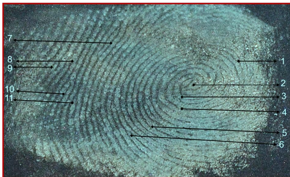
Fig.17. Latent fingerprints stained by \text{YAlO}_3:\text{Sm}^{3+} (1 mol %) nanophosphor for analysis of correspondences.
