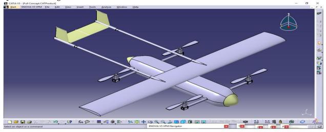
The quad configuration shows greater stability than both the bi and tri rotor configurations to achieve tilt rotor mechanism. Increasing the no of rotors directly increases the stability of the aircraft. However the quad configuration gives the desired stability and performance for the required weight considerations.
