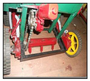
Figure 2.4.2: Digging Tool Arrangement
