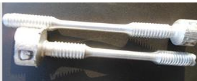
Fig. 5. Machined Tensile Specimen
