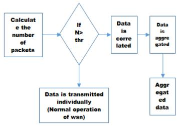
Fig4: Node-level data aggregation and correlation
