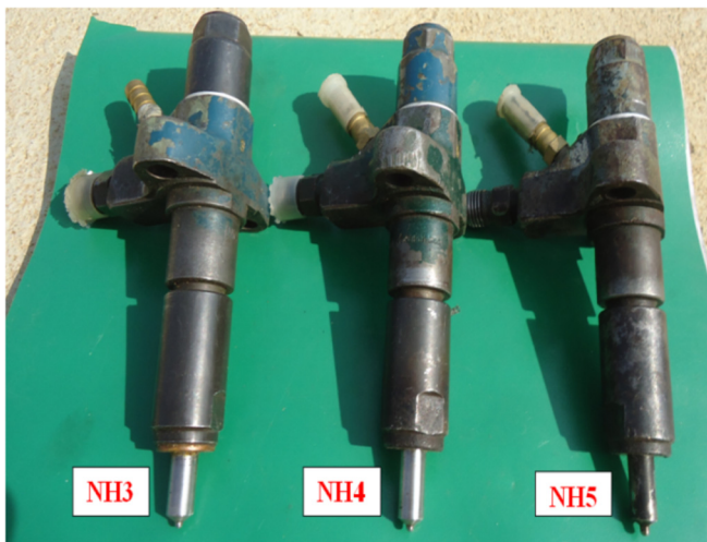
Fig. 4. Photographic view of 3, 4 and 5 holes nozzle fuel injectors.
