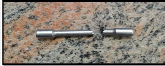
Figure.6.2.2 Specimen after tensile test
