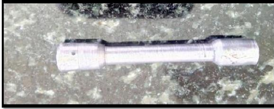
Figure.6.2.1 Specimen before tensile test
