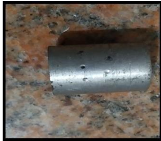
Figure.6.1.2 Specimen after hardness test
