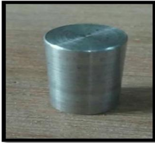
Figure.6.1.1 Specimen before hardness test
