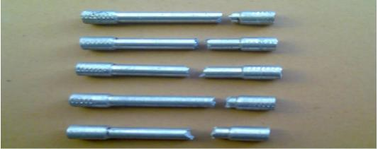
Fig. 2. Composite specimens after tensile test
