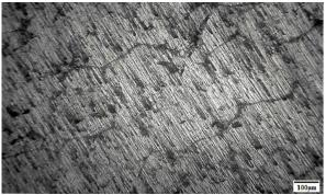
Fig. 9. Optical micrograph of worn sample of matrix alloy reinforced 4% flyash, 6% SiC at 15N load
