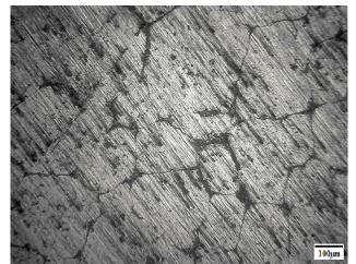
Fig. 10. Optical micrograph of worn sample of matrix alloy reinforced 4% flyash, 6% SiC at 20N load
