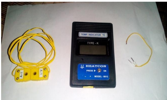
Fig 1: Thermocouple with Temperature Indicator
