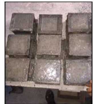
Fig. 2: Cube casting of NSC
