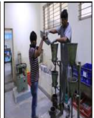
Fig.8: Compaction factor testing for NSC
