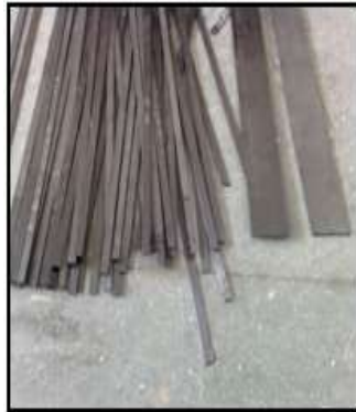
Fig 11: CFRP Laminates cut into strip
