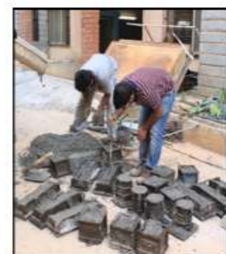
Fig.9: Casting of cubes, cylinders and prisms
