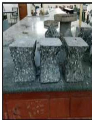
Fig.4: Failure of HSC cubes
