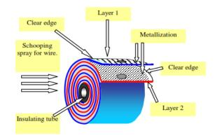
Fig.4: Normal spiral wound construction of cylindrical low power MKP capacitor using two vacuum metalized polypropylene strips.
