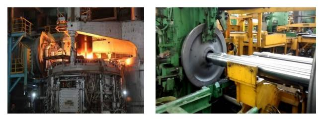
The wheels on easing go through the heat treatment process to develop optimum physical and metal logical characteristics. Each wheel is subjected to rigid international standards of quality control, including magnanimous and ultrasonic tests.
