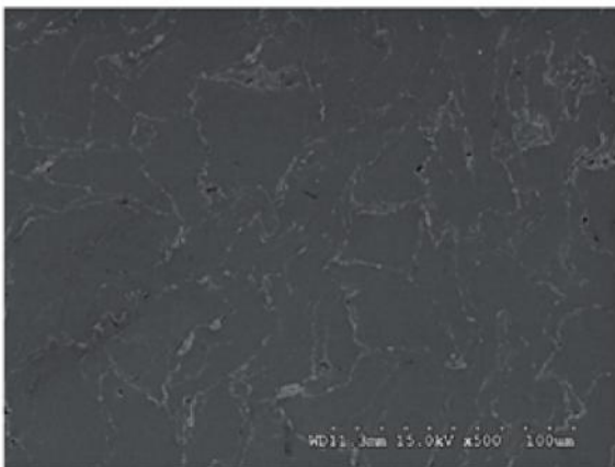
Figure 6: SEM Micrograph Showing Distribution of Al_2O_3 in Mg/1.0 Al_2O_3
