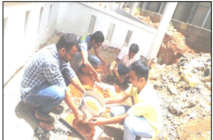
Fig. 2.1: Preparation of Sorbent Media Using Bricks
