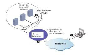
Load balancers are generally grouped into two categories: Layer 4 and Layer 7. Layer 4 load balancers act upon data found in network and transport layer protocols (IP, TCP, FTP, UDP). Layer 7 load balancers distribute requests based upon data found in application layer protocols such as HTTP. Requests are received by both types of load balancers and they are distributed to a particular server based on a configured algorithm. Some algorithms are:
