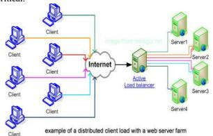
The proliferation of servers for various applications has created data centers full of server farms. One must ensure scalability and high availability for all components, starting from the edge routers that connect to the Internet, all the way to the database servers in the back end. Load balancers have emerged as a powerful new weapon to solve many of these issues.
