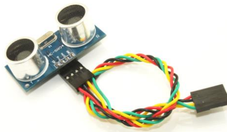
Figure 3. HC-SR04 Ultrasonic Module
