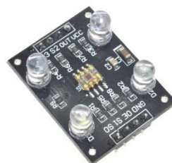
Figure 2. TCS230 RGB Color Sensor Module
