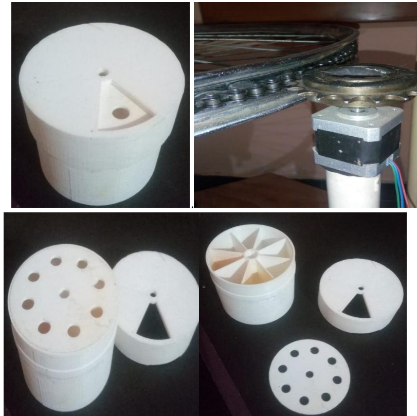
Fig 4.2 Testing the ingredient dispenser and therefore the wheel that carry dispensers.
