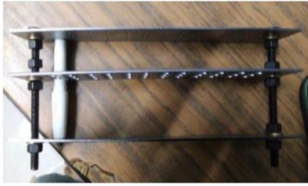
FIG 7: CAM FOLLOWER ASSEMBLY AND HOLDER
