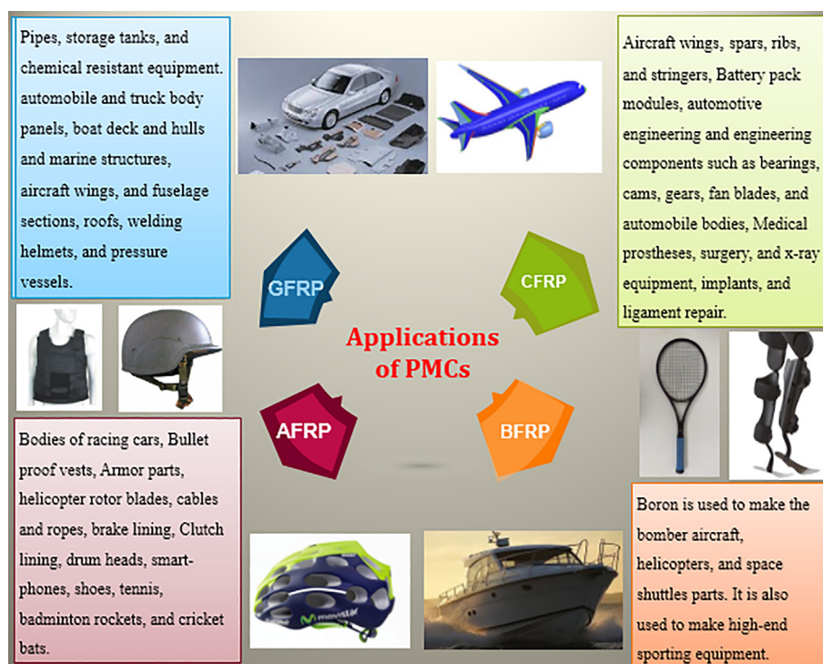
Fig. 9. Real time application of different fiber-reinforced composites.
