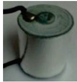
Fig. 2: Capacitor element ready for oil impregnation
