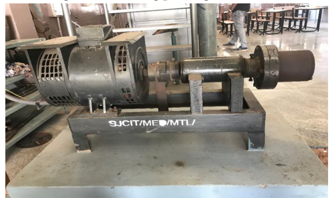
Fig 2: Centrifugal Casting Machine
