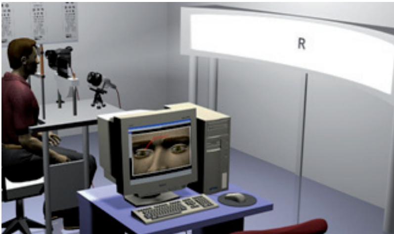
Figure 12. Video-Oculography used in DVA. It describes the subject position, Video camera matched to a PC to record the video, optotype and screen of projection.
