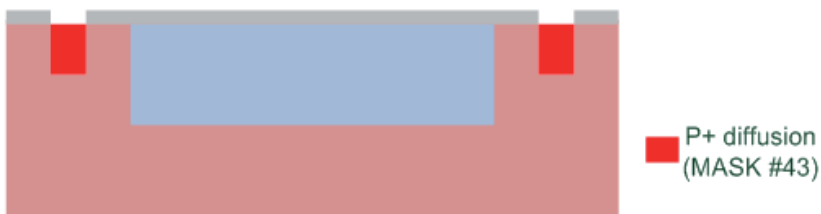
Figure 14. Guard ring get with P+ diffusion.
