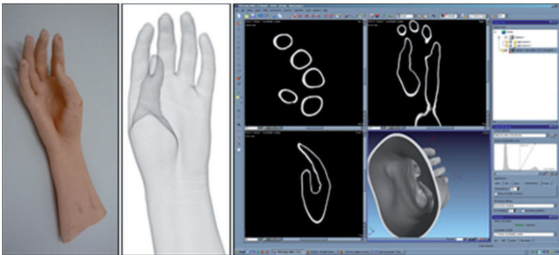
Figure 10. Epithetic hand glove (left), its X-ray scan (middle) and an environment of the VG-Studio Max software with three cross-sections and 3D view of rendered model of the glove.
