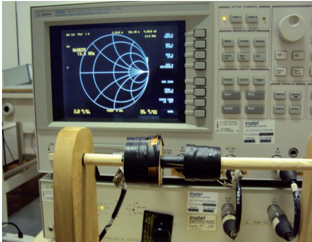
Figure 16. Free space measurement test set up.
