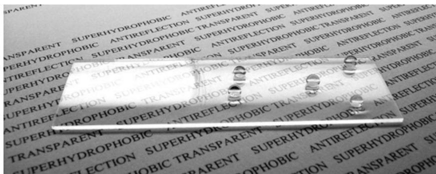
Fig. 9. Image of a glass slide coated with a transparent, superhydrophobic multilayer with antireflection properties (Bravo et al. 2007). (Reproduced with permission from the American Chemical Society, Copyright 2007.)
