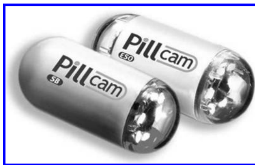
Figure 16.11 Given Imaging's capsule endoscope for small bowel (left) and esophageal (right) imaging. (Courtesy of Given Imaging.)
