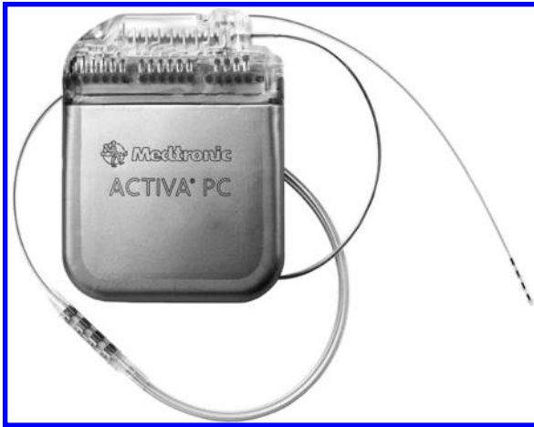
Figure 16.2 Hermetic titanium housing containing an implantable pulse generator (IPG) connected to a four-electrode pacing lead that is implanted in the brain for the treatment of Parkinson's disease. (Courtesy of Medtronic, Inc.)
