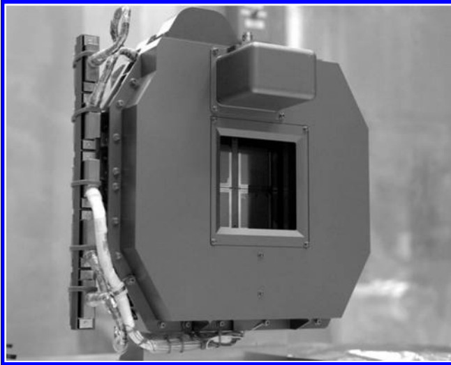
Figure 6.6 The Near-Infrared Spectrograph (NIRSpec) microshutter assembly. (Courtesy of the National Aeronautics and Space Administration.)
