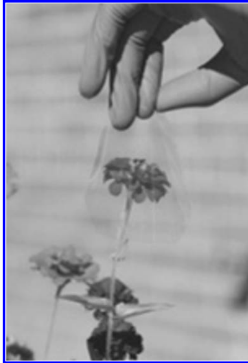
Figure 8.16 Transparent cured bionanocellulose composite in front of a flower at the Johns Hopkins University's Applied Physics Laboratory (JHU/APL). Sample thickness was measured to be 110 \mu\text{m} .
