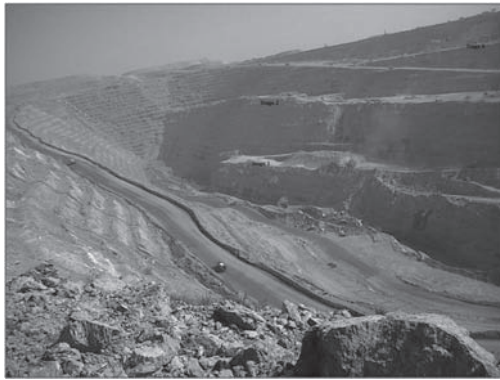
Figure 1. Rampura Agucha open pit showing various stages of excavation on hangwall.
