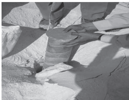
Figure 3. View of the bottom air deck technique.
