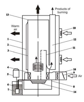
Figure 4. Gasgenerator which works on exhaust fuel: 1 - corps; 2 - pipe; 3 - combustion chamber; 4 - mixer; 5 - an electric motor; 6 - tank with fuel; 7 - pump; 8 - pallet; 9 - bolt; 10 - ventilator; 11 - screen; 12 - place of gas moving; 13 - lid; 14 - plate.
