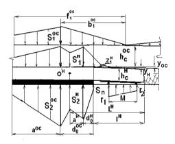
Figure 1. Design model to calculate stress-strain state of roof stone rocks.
