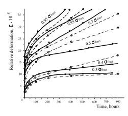
Figure 1. Curves of Gypsum Creep
