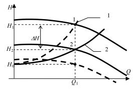
Figure 6. Q-H curves for regulation under various supply.
