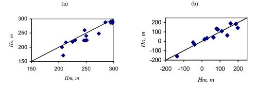
Figure 6. Comparison of modeled (Hm) and observed (Ho) ground water heads: (a) second layer, (b) fourth layer.
