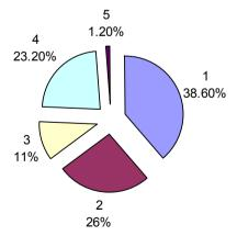
Figure 5. Calculated balance components of water inflow to mine in 1990: 1 – recharge, 2 – storage, 3 – shortening of ground water runoff, 4 – surface water inflow, 5 – shortening of infiltration.
