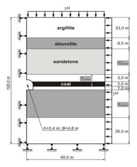
Figure 5. The generalized solution scheme.
