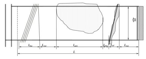
Figure 2. Design diagram for determination of deposits produceability in extraction panel.
