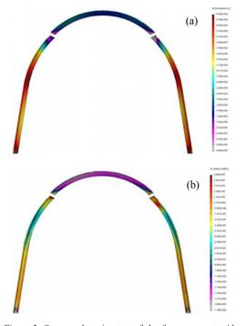
Figure 3. Stress and strain state of the frame support with simulators of the yield locks: (a) distribution diagram of calculation stresses  $\sigma$ ; (b) distribution diagram of horizontal stresses  $\sigma_x$ .
