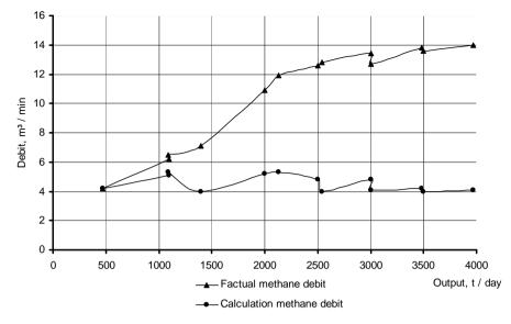
Figure 2. Dependence of methane distribution in workings on coal production rate.
