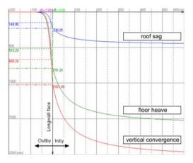
Figure 14. Results of computations of the course of gateroad convergance outby and inby the face based on empirical method worked out at GIG (Prusek 2007).
