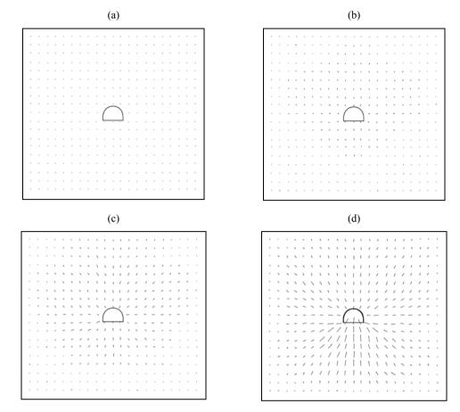
Figure 3. Vectors of angular points displacement on measured grid for homogeneous model at loadings: (a) 0.00 kN, (b) 2.61 kN, (c) 4.56 kN, (d) 7.04 kN.
