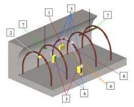
Figure 16. Scheme of monitoring system of roadway support: underground computer (1), module for support deformation measurement by means of the photogrammetric method (2), laser module (3), hydraulic dynamometers (4 and 5), displacement sensors to measure the slide in support friction joints (6), tensometric sensors to measure the force acting at the support shackles' bolts (8). – (Prusek 2008b).
