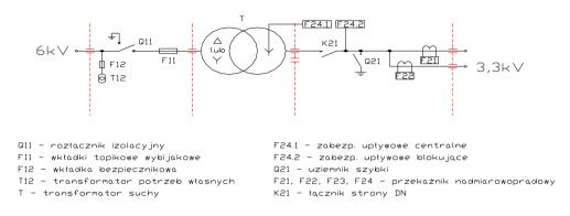
Figure 2.1. Schematic (one-wire) diagram of the transformer station type EH-d31-2600/6,0/3,3/02.01.
