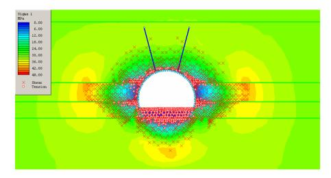
Figure 2. Volume of plastic zone around Cw-1 heading.
