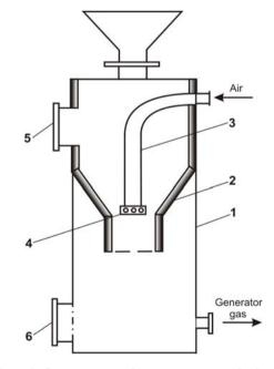
Figure 3. Gasgenerator on the generator gas production: 1 – metallic corps; 2 – cone; 3 – pipe; 4 – snuffled the air serve in the burning zone; 5, 6 – air-tight doors.
