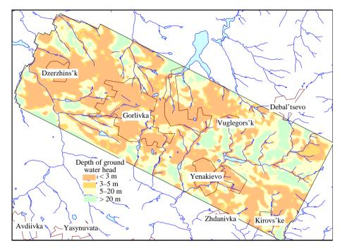
Figure 4. Depth of ground water head before mining calculated by modeling.
