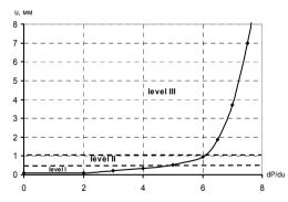
Figure 2. Dependence of floor heaving on the intensity of an exterior loading.
