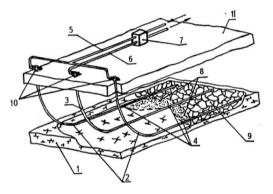
Figure 1. Technological scheme of underground coal gasification from a surface: 1 – coal seam; 2 – injection wells; 3 – production well; 4 – movable ignited devices; 5 – air pipeline; 6 – gas pipeline; 7 – heat – utilization; 8 – combustion face; 9 – goaf; 10 – adjutage of the directed boreholes; 11 – surface.
