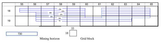
Figure 3. The mine works schedule on the mine named after Rumiantsev over the seam "Yulievs'ky" according to gridding.
