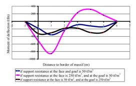
Figure 4. Lines of behaviour of moments of deflection along the length of roof stone.
