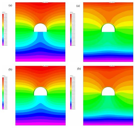
Figure 3. Distribution diagrams of displacements in system "stratified massif-support of working" at increased of strength and decreased of deformation characteristics of all adjacent rock layers: (a) H = 200 m; (b) H = 600 m.
