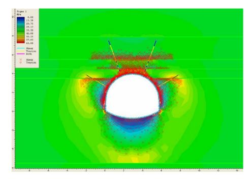
Figure 4. Plastic zone around the cross heading.
