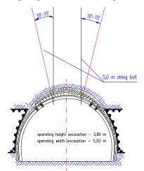
Figure 1. Support scheme for Cw-1 heading.
