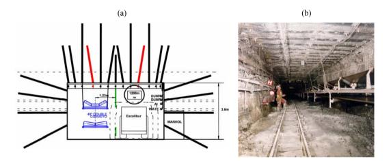
Figure 4. Rock bolted gateroad in one of the UK mines; (a) detailed scheme of rock bolting, (b) view of rectangular rock bolted gateroad.
