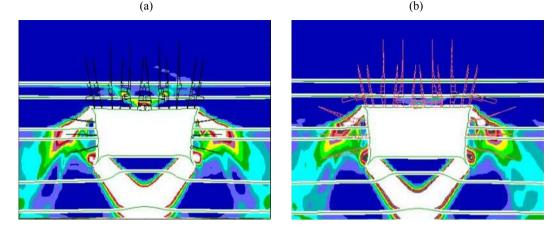
Figure 11. Numerical modeling of gateroad deformation at Daw Mill Colliery; (a) conventional scheme of bolting; (b) scheme of bolting using side wall rock bolts with increased length and diameter (Bowler, Robinson & Altounyan 2009).
