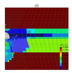
Figure 6. Configuration APD: (a), (c), (e) up to the floor heaving; (b), (d), (f) after the floor heaving, I – homogeneous rock mass including a coal seam; II – rock mass including a coal seam and seam of sandstone in roof (distance between coal seam and sandstone is  $h_{sandstt} = 10.0$  m); III – rock mass including a coal seam and seam of sandstone is floor (distance between coal seam and sandstone is  $a_{sandst} = 7.0$  m).
