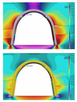
Figure 2. Stress and strain state of the system "rock massifsupport" with full reflection of the yield lock's structure: (a) distribution diagram of calculation stresses  $\sigma$ ; (b) distribution diagram of horizontal stresses  $\sigma_x$ .
