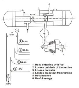
Figure 2. Scheme of equipment situate and power diagram of engine with free pistons.
