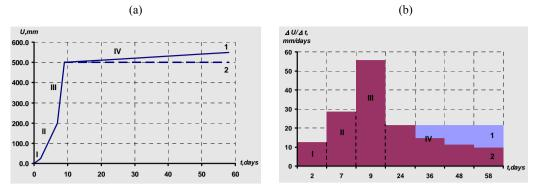
Figure 1. Displacements (a) and speeds of displacements (b) of contour with in meters of "Belozerskaya" of "Dobropol'eugol" (1 – undamping process and 2 – damping process).
