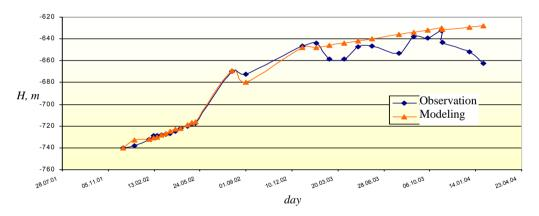
Figure 7. Rise of ground water head H in coaly rocks during flooding of the mine "Chervony Profintern".
