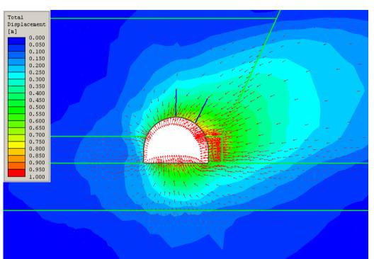
Figure 15. An example of numerical modeling of the rock mass around gateroads; (a) zone of rock mass damage in the surroundings of the gateroad, axial forces and vectors of support displacements at a distance of 54 m inby the face (Prusek & Masny 2007), (b) displacements of rock strata into the gateroad at a distance of 100 m inby the face (Prusek 2008c).
