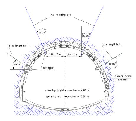
Figure 3. Scheme of cross heading's full support.
