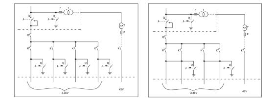
Figure 2.2 (a). The schematic diagram of the four-outlet contactor switch of the type EH-W/3,3/I/01.xx and the schematic diagram of the contractor switch type EH-d03-W/3.3/I/02.xx intended for reversible supply of main motors intended to drive the coal plough.
