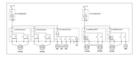
Figure 2.2 (c). The schematic diagram of the power supply system for the high-performance longwall set of equipment operated in the Hard Coal Mine "Zofiówka".
