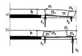
Figure 3. Behavior of stress condition of roof stone.
