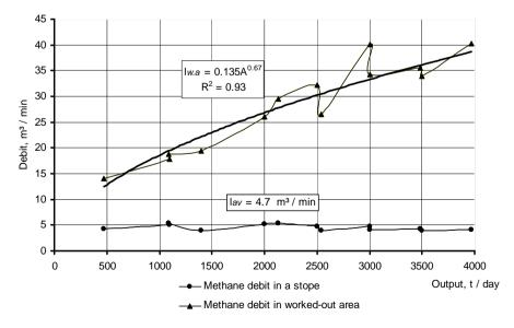
Figure 1. Dependence of methane debit in a stope on coal production rate.
