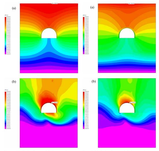
Figure 1. Distribution diagram of displacements in system "stratified massif-support of working" at decreased strength and deformation characteristics of all adjacent rock layers: (a) H = 200 m; (b) H = 600 m.
