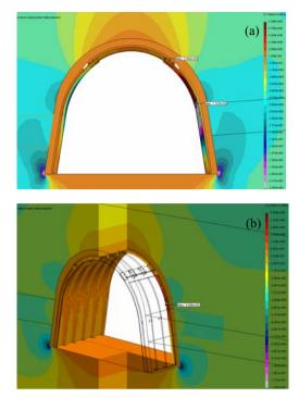
Figure 1. Stress and strain state of the system "rock massifsupport" with full reflection of the yield lock's design: (a) distribution diagram of vertical stresses  $\sigma_y$ ; (b) distribution diagram of axial stresses  $\sigma_z$ .
