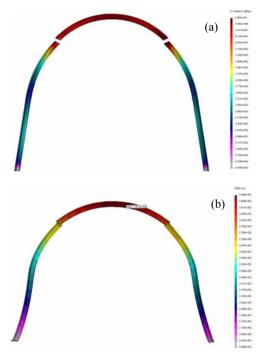
Figure 4. Stress and strain state of the frame support with simulators of the yield locks: (a) distribution diagram of vertical stresses  $\sigma_y$ ; (b) distribution diagram of full displacements U.
