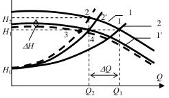
Figure 2. Regulation under constant pressure.
