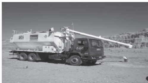
Figure 13. PANFO truck used at Esperanza Mine trials.
