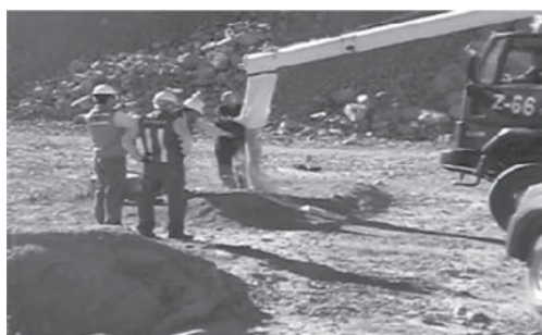
Figure 14. Discharging PANFO into a blasthole.
