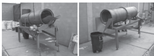
Figure 8. Rotating trommel used to screen Perlite dust & fines.
