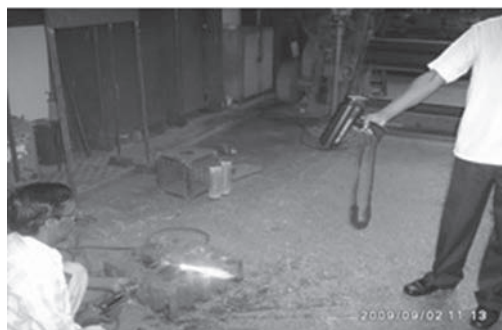
Figure 6. Measurement of temp. by IR Pyrometer.
