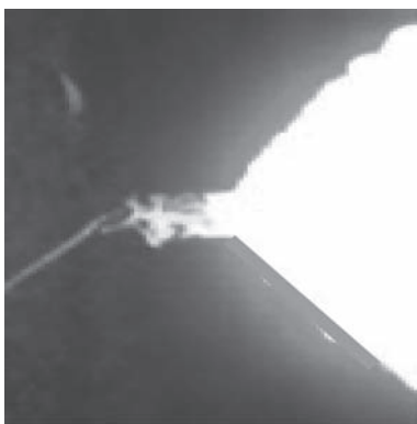
Figure 11. Expansion of detonation products of emulsion in pipe (note pipe was actually vertical).
