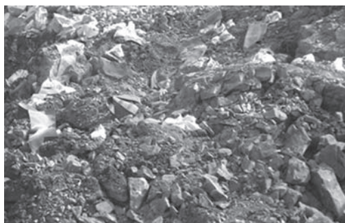
Figure 5. ANFO blast result in jointed fractured sandstone overburden coal mines.
