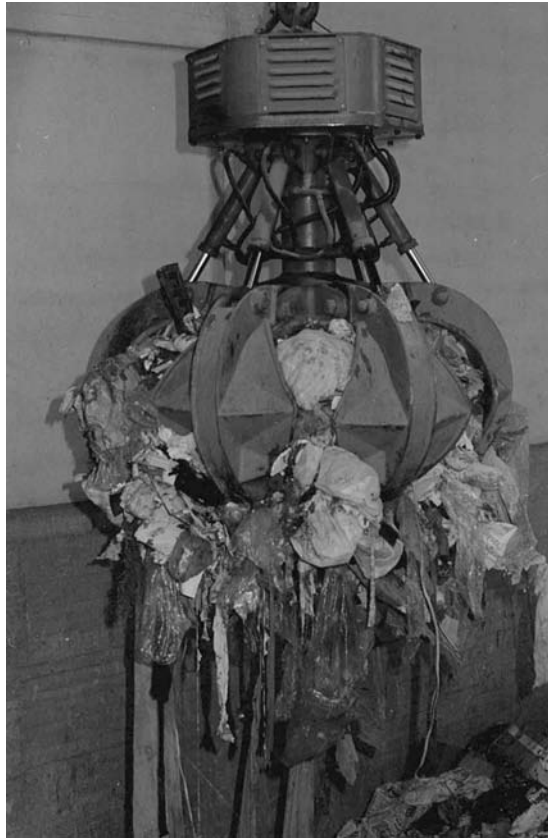
FIGURE 8.6 Orange peel type MSW bucket. (Courtesy of Gensco equipment.)
