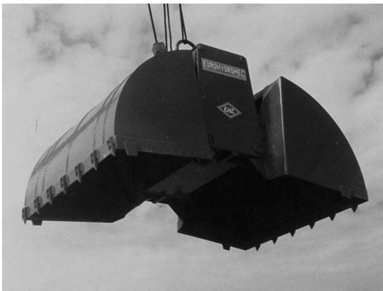
FIGURE 8.4 Clam shell type MSW bucket. (Courtesy of Gensco equipment.)
