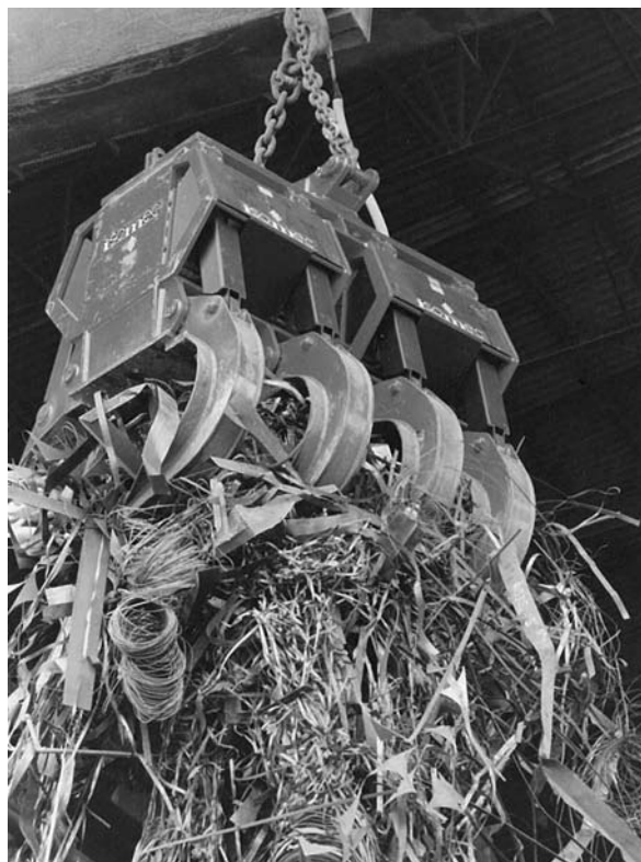
FIGURE 8.5 Grapple type MSW bucket. (Courtesy of Gensco equipment.)
