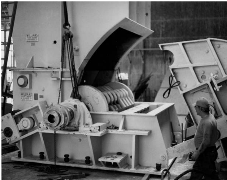
FIGURE 7.3 Horizontal shaft hammermill for refuse processing. (Courtesy of Williams Patent Crusher & Pulverizer Co., Inc., St. Louis Missouri www.williamscrusher.com .)
