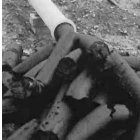
FIGURE 7.12 Extruded high solids sludge from piston pump. (Courtesy of Schwing Bioset, Inc.)
