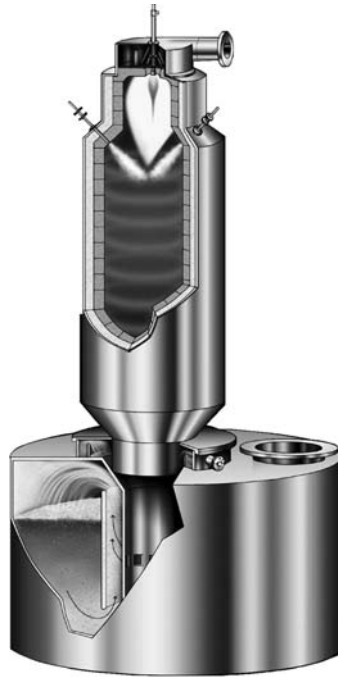
FIGURE 10.2 Sub-X system for high salt content wastes. (Courtesy of Selas Fluid Processing Group.)
