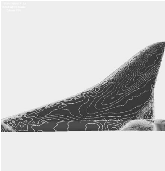
FIGURE 7.14: Flow around Dassault SSBJ geometry, Mach 1.6, incidence 0: Mach number contours on upper side obtained by applying the new version of the scheme.
