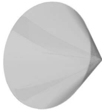
FIGURE 7.16: Left: global mesh convergence order for the SSBJ: a second order spatial convergence is obtained. Right: the Mach cone emitted by the SSBJ. The maximal Mach cone diameter is 1.25 kilometers.
