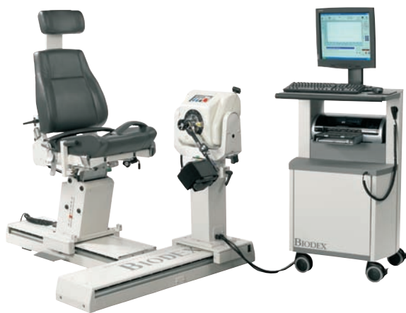
Figure 4.2 An example of an isokinetic exercise and testing unit. Isokinetic dynamometers may be used for testing and exercising muscle groups isokinetically, isometrically, concentrically, or eccentrically. Depending on the specific unit, force or torque exerted by the muscle group is recorded along with joint angles and motion. The computer provides calculations for average peak torque, work, and power.
