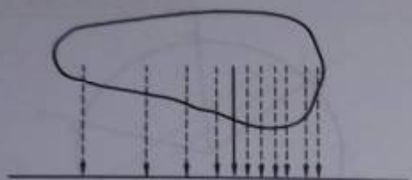
Fig. 8.14 The line of gravity of an object (solid arrow) is a line along which the whole weight of the body may be considered to act, although each part of the body has weight (dashed arrows).
