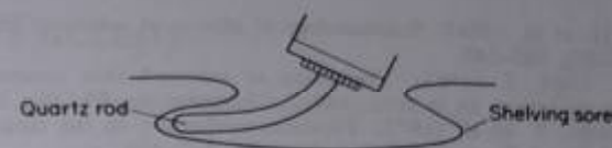
Fig. 6.8 A quartz rod applicator may be used with the Kromayer head for the treatment of a shelving sore or a sinus.
