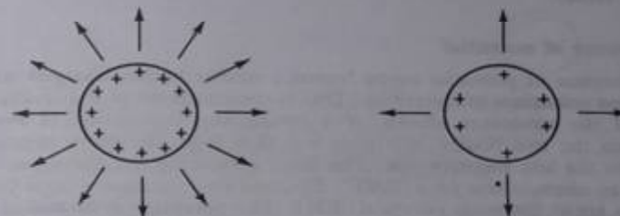
Fig. 1.8 The greater the charge, the greater the potential (repelling power) of a charged object.
