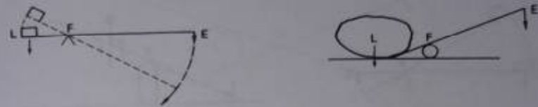
Fig. 8.25 First-order levers with a long effort arm and hence a mechanical advantage.
