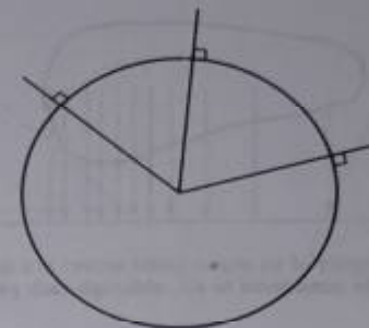
Fig. 8.13 A line passing through the centre of a circle is perpendicular to the circle where it cuts it — hence gravity acts at right angles to the earth's surface.
