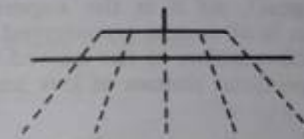
Fig. 4.18 A monopolar electrode producing a radial electric field.
