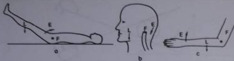
Fig. 8.30 Levers in the human body: (a) Flexion of the hip joint: third-order lever. (b) The skull balanced on the atlanto-occipital joint: first-order lever. (c) The action of the brachioradialis muscle as a flexor of the elbow; second-order lever.
