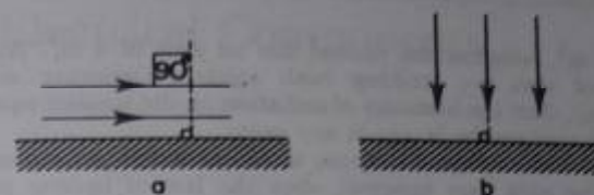
Fig. 1.31 (a) Angle of incidence = 90^\circ : no rays are absorbed. (b) Angle of incidence = 0^\circ : absorption is maximized.
