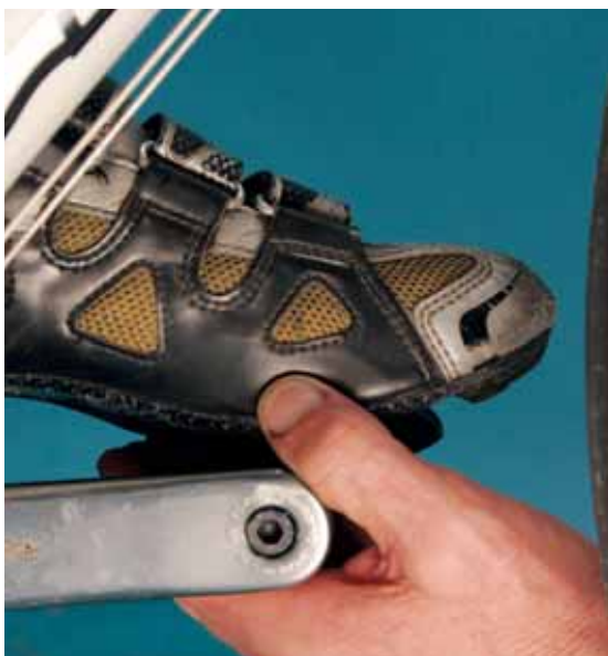
Figure 5.35 (a) Cleat position. Note the therapist's thumb is over the base of the first metatarsal, which lines up with the center point of the pedal spindle
