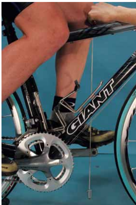
Figure 5.33 Measurement of seat fore/aft position: plumb bolt over axis
