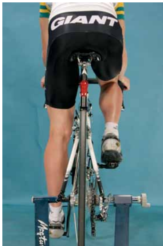
Figure 5.36 Seat width. Note how the narrow seat allows the cyclist's legs to drop down unimpeded
