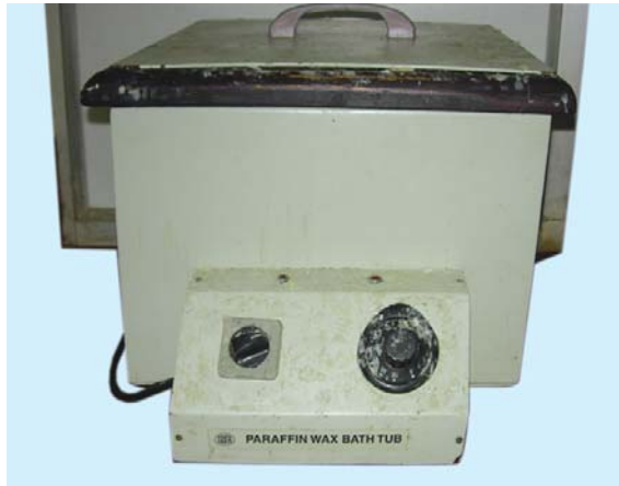
Fig. 1.8: Showing paraffin or wax bath equipment
