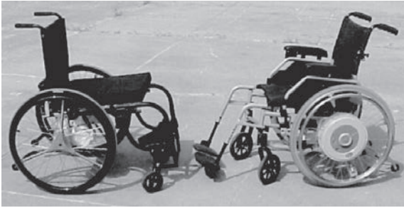
Fig. 23-9. Two power-assist wheelchairs. On the left, a prototype of a variable ratio power-assist wheelchair. On the right, the batteries and motor are in the hub of the wheel. (Illustration courtesy Charles E. Levy, MD.)
