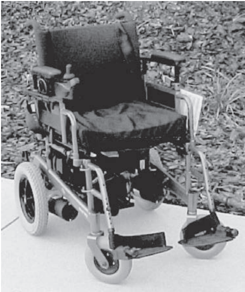
Fig. 23-6. A folding frame rear wheel drive power wheelchair. (Illustration courtesy Charles E. Levy, MD.)
