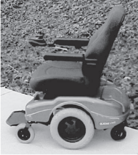
Fig. 23-7. A midwheel or center-wheel drive power chair. (Illustration courtesy Charles E. Levy, MD.)
