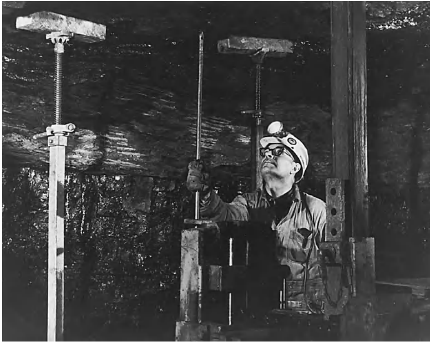
Figure 57-1 Roof bolting in underground coal mine. A potentially high-risk operation for respiratory exposures to airborne silica. (Photo courtesy of U.S. Bureau of Mines.)
